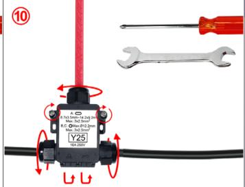
**9**: Insert the stripped part of the power supply conductors into the terminals and tighten with a screwdriver. 2 conductors inside each terminal, on each side of the saddle. Recommended tightening torque 1.2Nm.
